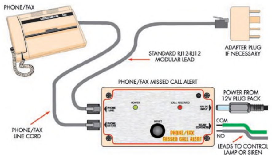
Fig.4: here's how to connect it to the phone line. At left are shots of the drilled case lid and the completed assembly going into the case.
