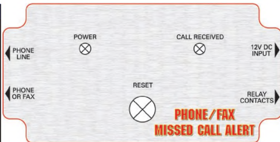
Fig.5: above is the same-size front panel artwork (also useful as a template!) while the PC board pattern is shown below.
