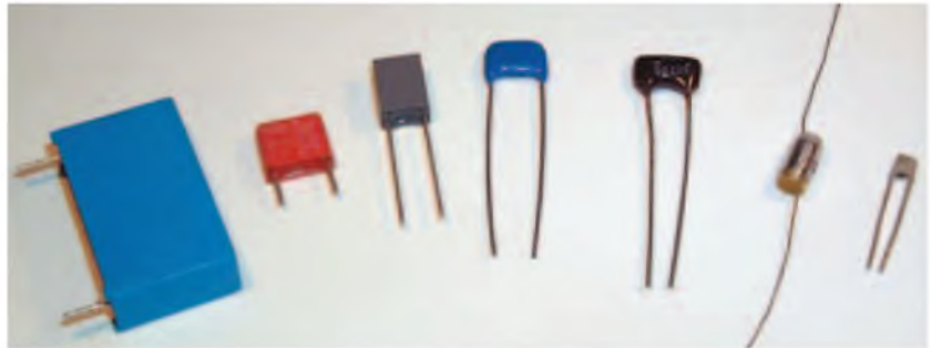
Fig.3. Various non-electrolytic capacitors with values ranging from 1pF to 470nF and voltage ratings from 50V to 250V
