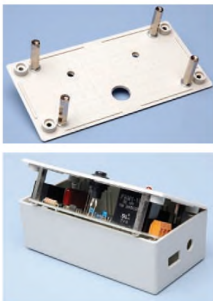
Fig.4: here's how to connect it to the phone line. At left are shots of the drilled case lid and the completed assembly going into the case.
