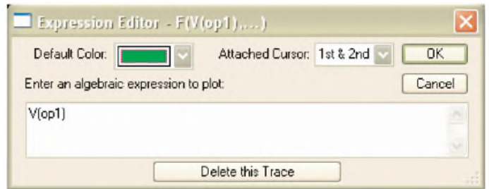
Fig.3. Setting up cursors on the output waveform
