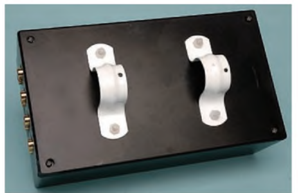
The two saddle clamps are held in place with nylon screws and nuts to prevent shorts.
