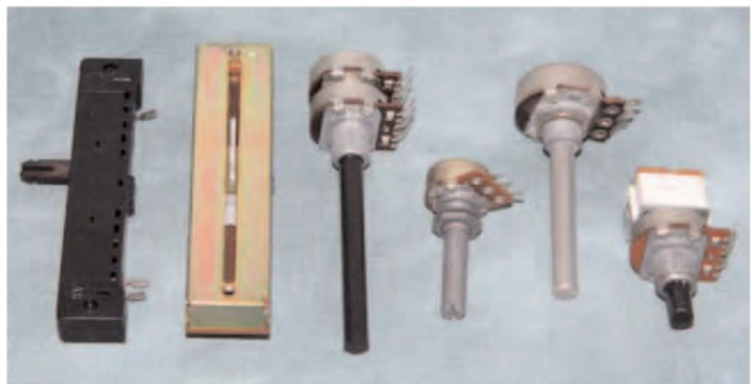
Fig.1. Potentiometers are available in various styles as well as in a range of different values. They are also relatively expensive
