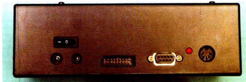
End-on and side-on views showing the eight inputs (left); above is the DC in/out, games port socket, serial socket, invalid MIDI LED and MIDI output
