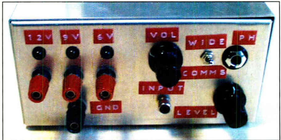
Fig.2: General layout of front panel components
