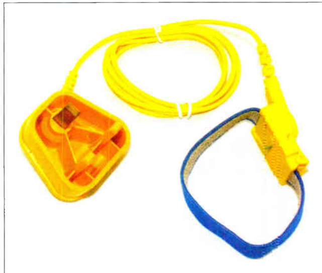
Fig. 2. A conductive wristband connects to the mains earth via a lead that has a high series resistance, and a special (safe) form of mains plug
