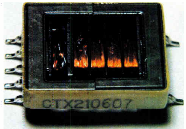
Fig.5. Transformer suitable for use with Royer converter circuit
