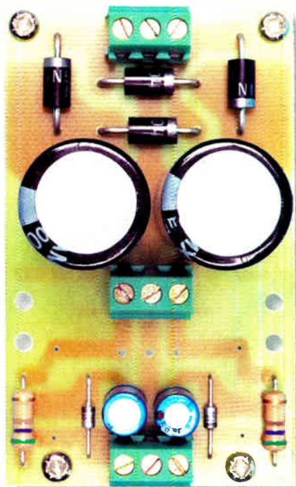
This view shows the completed power supply for the amplifier. The components at the bottom are for the optional ±15V preamp power supply and may be left out if not required.
