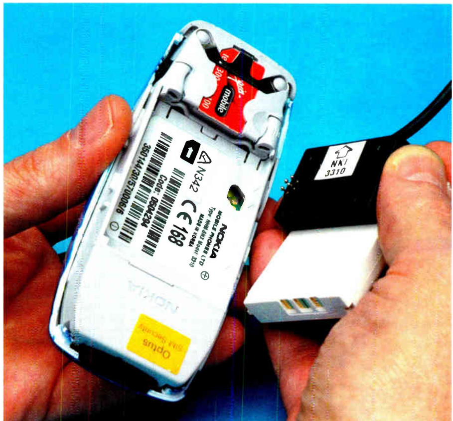
On the 3310 model, the serial interface is accessible through a hole in the rear of the case, underneath the battery. The data cable is terminated with a plastic head assembly that includes a set of spring-loaded contacts as well as tabs to retain the battery that it partly displaces.
