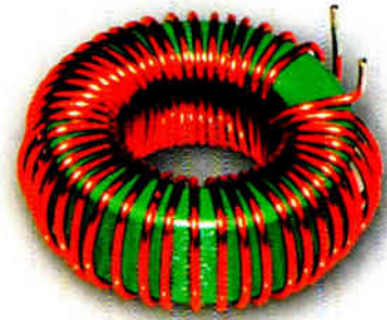
Bend and shape the ends of the winding so that the assembly slips easily into the holes in the PC board. This shot of the underside of L1 shows the general idea, although this core doesn't have the full 50 turns!
