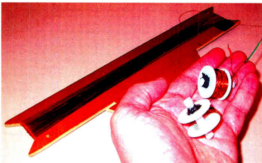
The homemade, power booster inductor is made up from a plastic bobbin and 60 metres of 36swg (32awg) enamelled copper wire. The wire was measured out using a half-metre wooden former.
