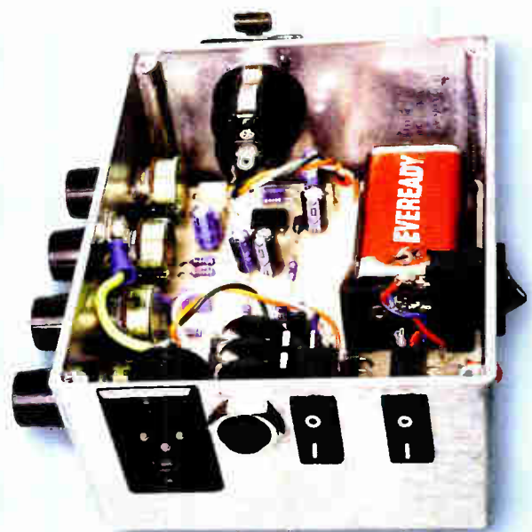
Right: this end of the case carries (from left to right) the 3-pin male XLR socket (CON3), a 6.5mm jack socket (CON2), the Ground Lift switch (S2) and the Power switch (S1). The 3-pin female XLR socket mounts on the other end of the case
