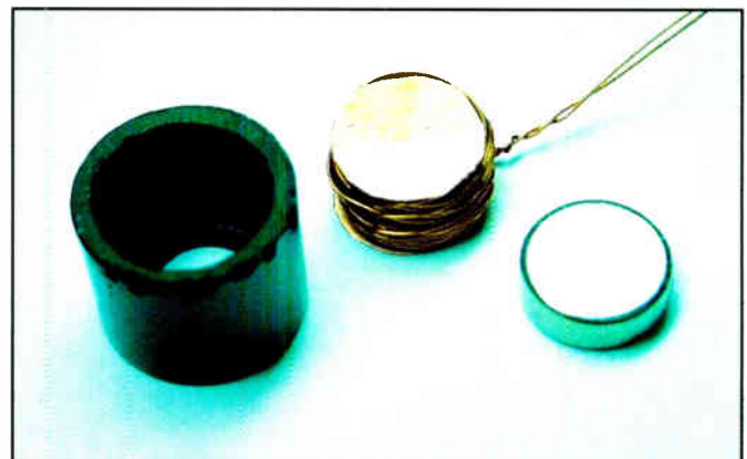
Component parts that make up the electromagnet. Left to right: trimmed plastic barrel of a 5mm jack plug, coil assembly and a 9mm diameter neodymium magnet
