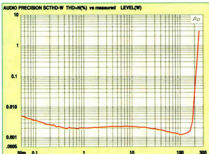
Fig.2: total harmonic distortion versus power at 1kHz into an 8-ohm load (10Hz-22kHz measurement bandwidth).
