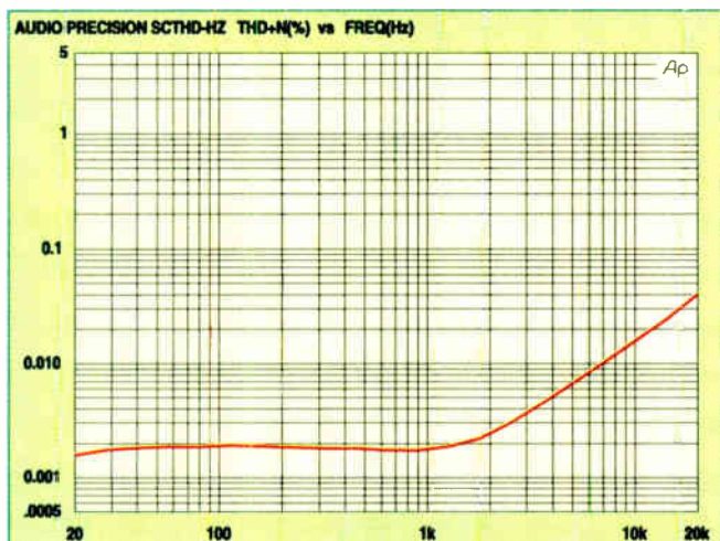
Fig.4: harmonic distortion versus frequency at 160W into an 8-ohm load (22Hz-80kHz measurement bandwidth).
