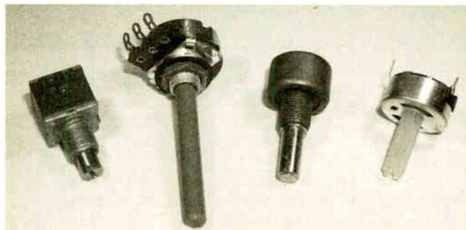
Photo 1.3. Various types of rotary potentiometer. From left to right: miniature wirewound, carbon track rotary, wirewound, carbon track with p.c.b. mounting tags
