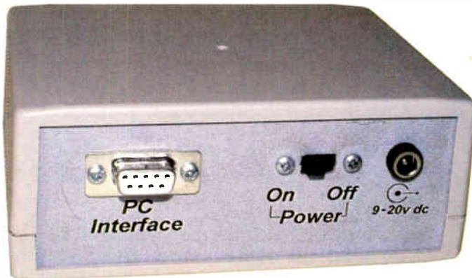
Front and rear views of the Speed Camera Watch Mk2. The function buttons (S2 to S5) are mounted either side of the front panel display window. The PC Interface socket is located on the back panel as indicated
