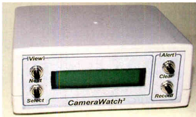
Front and rear views of the Speed Camera Watch Mk2. The function buttons (S2 to S5) are mounted either side of the front panel display window. The PC Interface socket is located on the back panel as indicated
