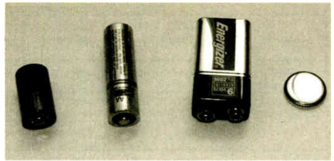
Photo 1.4. Various types of battery. From left to right: a 3V lithium (Li) battery, a 1.2V nickel-metal hydride (Ni-MH) cell, a 9V alkaline battery, a 3V lithium (Li) button cell
