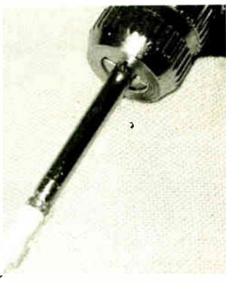
Fig.1. High drill speeds and most plastics do not go well together
