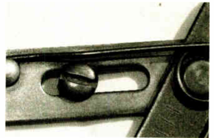
Fig.4 Loosening the bolt enables it to be slid to a new position and tightened again. This method of adjustment is fine if only occasional readjustment will be needed
