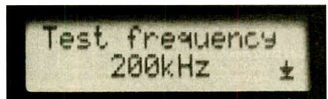
Pressing the Scroll-Off button displays the test frequency (200kHz) on the instrument's screen
