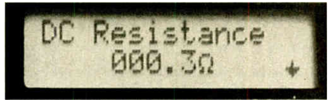
In this screen shot the d.c. resistance (0.3 \Omega ) of an inductor is displayed
