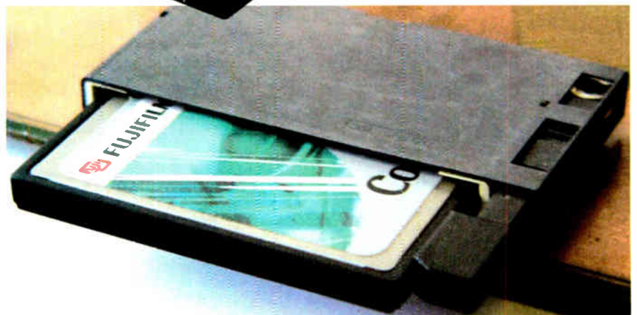
Photo 3 (below). CompactFlash card in header, with ejector mechanism
