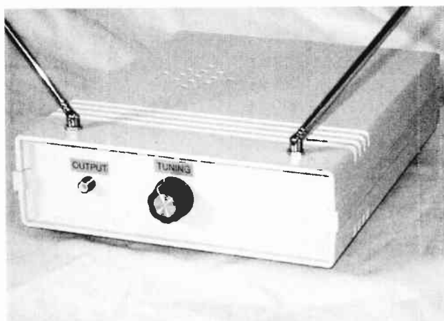
Rear view of the Theremin showing the phono output socket, tuning control (VR4) and sensor "aerials" mounting.
