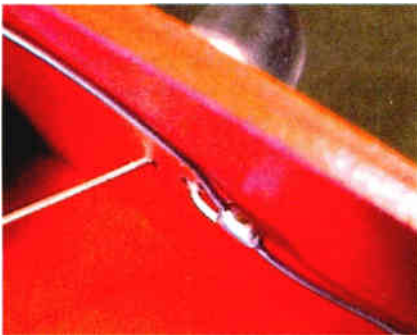
Running a common l.e.d. anode wire around the upper deck side panel.
