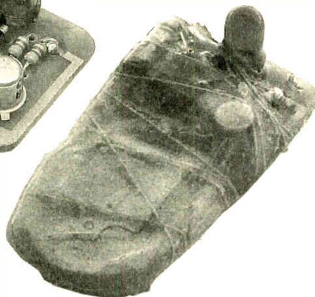
(Above) The "mummified" printed circuit board, including the lithium cell battery. (Right) Underside view of the p.c.b. The two large copper areas at the top left-hand corner are the "switch moisture contacts". These pads must not be covered with resin - see text.
