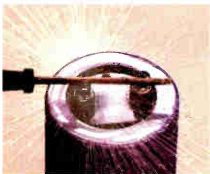
Photo 1.5. A dramatic (but dangerous) illustration that a capacitor stores electrical charge (see text).
