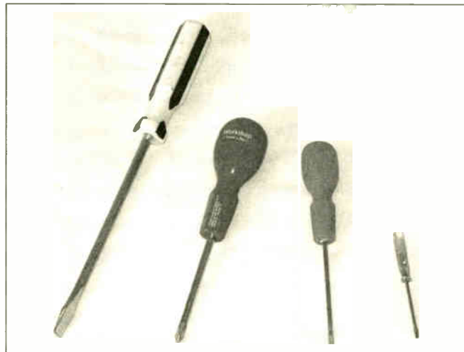
Fig.1. The large screwdriver on the left is the type found in most toolkits. The three smaller screwdrivers are what you need for project building.
