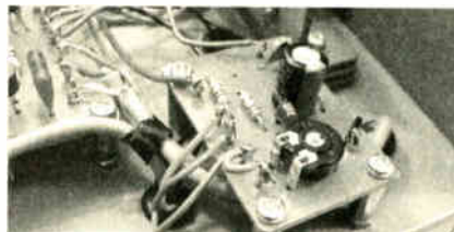
Fig.4.2. Printed circuit board component layout, wiring details and full-size underside copper foil master for the Varicap Tuner. Clockwise rotation of the pots. reduces the capacitance and increases frequency. The lead-off wires go to last month's Regenerative Radio.
