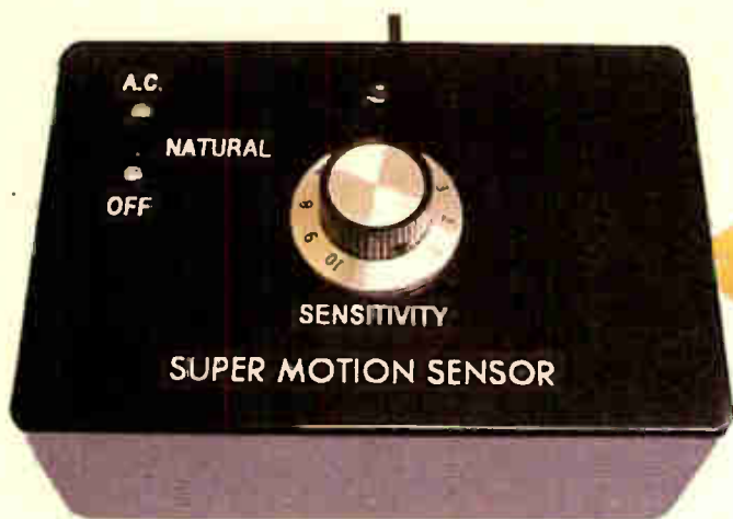
Completed Sensor showing front panel Sensitivity control and the lighting conditions slide switch.
