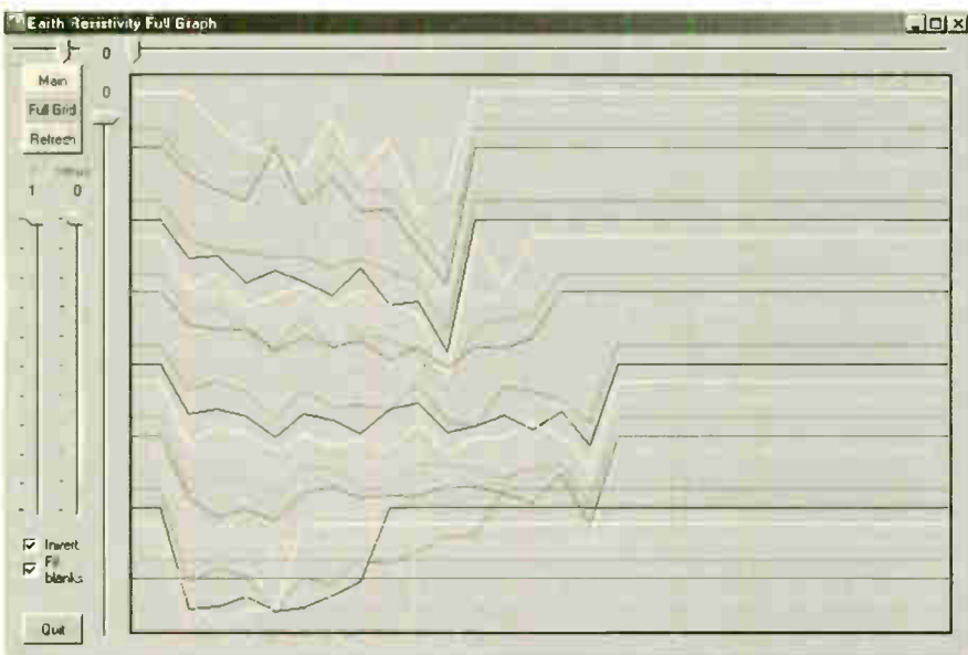
Example of the full screen graph display. The zoom is at x9 to emphasise the contour lines. The samples cover a maximum area of 16 rows x 26 columns, each sample representing one square metre. The data is the same as in the full grid display and is in eight colours on the screen.
