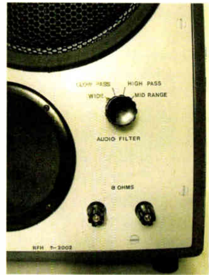
Crossover/Audio Filter selection switch and amplifier input terminals.
