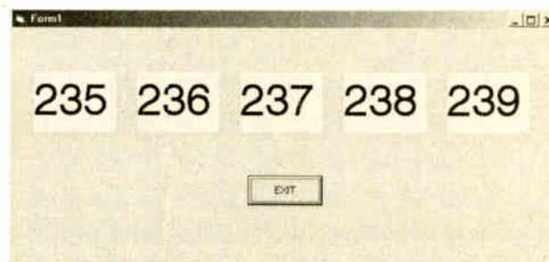
Fig.4. A group of five bytes have been displayed correctly. The transmitting program has started at 234 and then incremented five times so that values of 235 to 239 have been transmitted.
