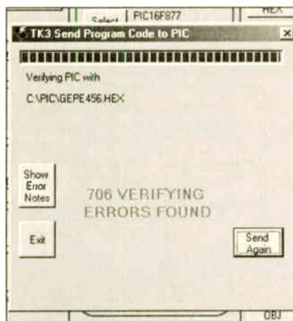
Photo 13. Programming sub-screen following detection of programming errors (image simulated for sake of illustration - you are unlikely to experience verification errors).
