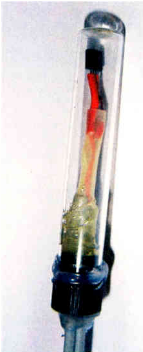
The LM35DZ enclosed in a sealed glass tube.
