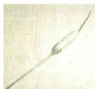
Large 3 amp 25 uh choke size 4.5 in long by 10 mm wide. Order No 38-0882 3 for £1
