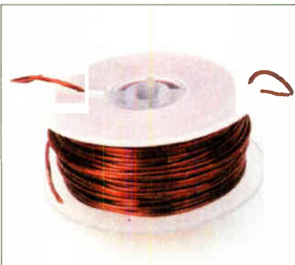
Loudspeaker crossover coil: Commercially produced 1mH loudspeaker crossover unit inductor. This air-cored coil has an outside diameter of 50mm and is 25mm long.
