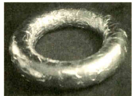
Toroidal discharge terminal.
