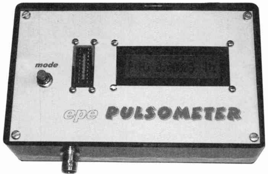
Finished PIC Pulsometer showing front panel display cutout and the 20-way d.i.l. socket for testing capacitors. The top half of the socket has been painted red to identify the "positive" side.
