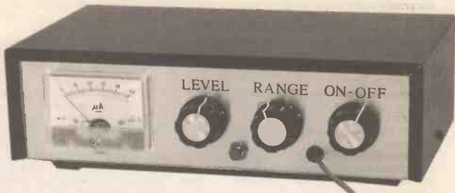
Finished unit showing front panel layout and lettering. Note the phototransistor/diode light sensor is attached to the free end of the screened cable.
