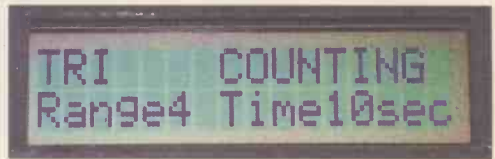
When the sampling rate change switch is pressed the word "counting" is displayed until the first new count has been completed. In this instance a 10-second sampling rate has been selected.
