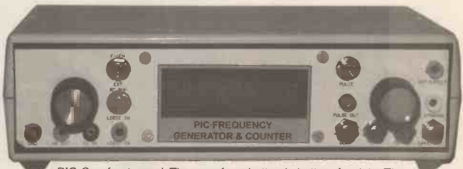
PIC-Gen front panel. The waveform button is bottom far right. The switch marked "pulse" (top right) is the on/off switch in the final model.
