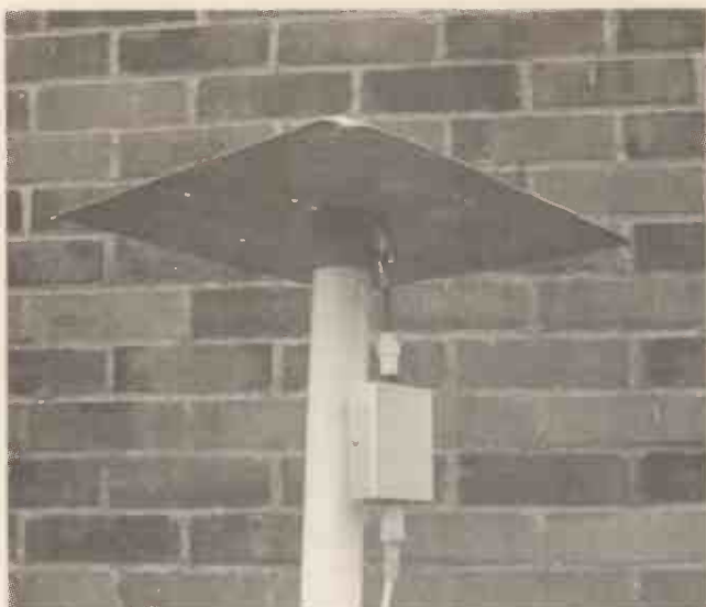
Meter interface unit connected to the sensor probe plate.
