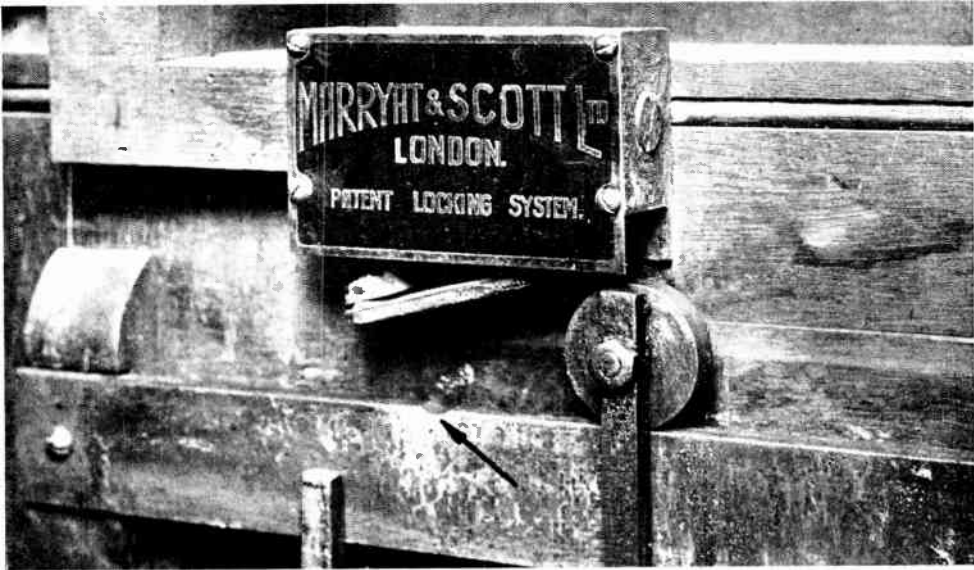
Fig. 5.—PREVENTING THE CAR GATE FROM VIBRATING OPEN.
