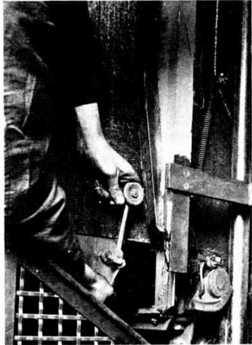
Fig. 3.—MAKING A FINE ADJUSTMENT ON THE CONTROL LIMIT SWITCH.
