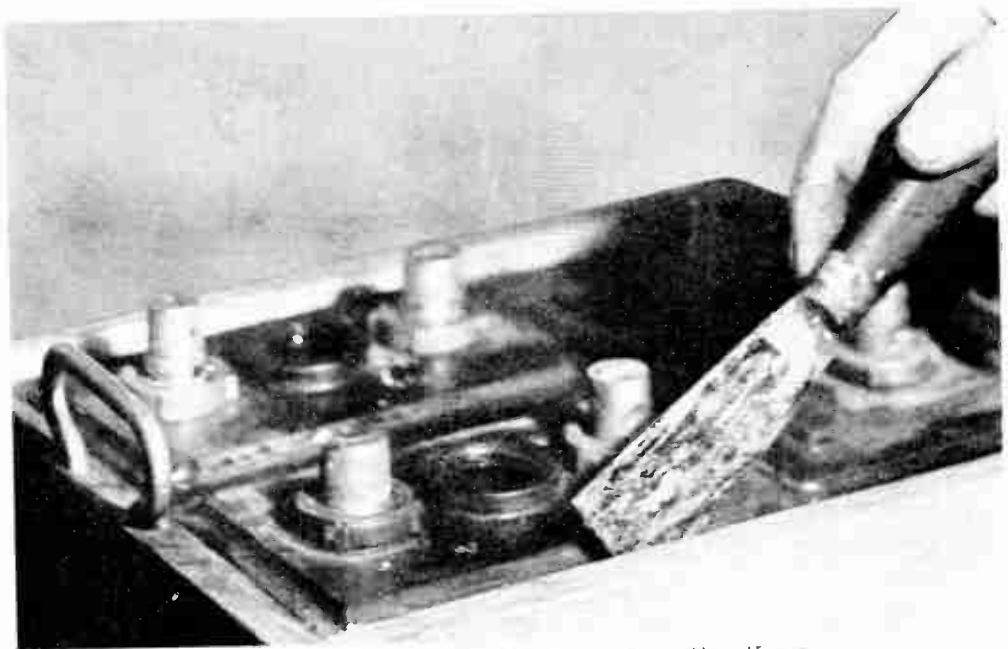
Fig. 1C. —REMOVING THE COMPOUND WITH A HOT KNIFE. This is done after the compound has been softened as shown in Fig. 1B.
