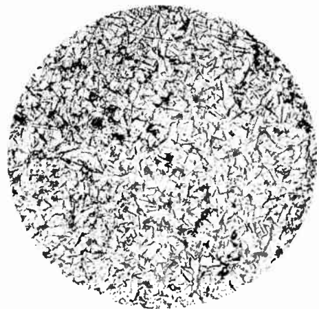
Fig. 17.—MICROGRAPH \times 100 SHOWING THE WELD METAL FROM FLUXED ONLY ELECTRODE.
