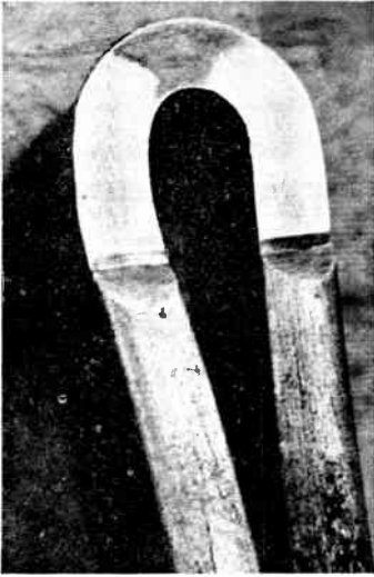
Fig. 10.—SHOWING HOW WELD METAL CAN BE DEPOSITED WHICH WILL ALLOW THE MAXIMUM COLD BENDING OVER A DIAMETER EQUAL TO THE WORK PIECE'S OWN THICKNESS.
