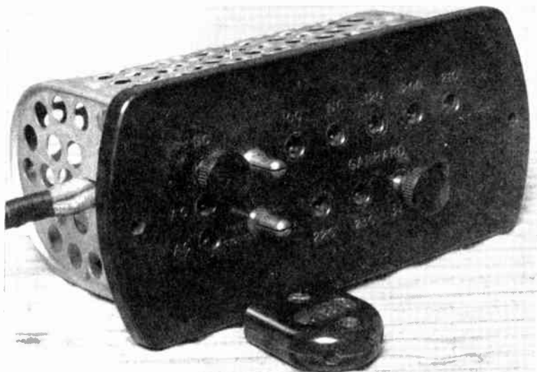
Fig. 4.—RESISTANCE FOR ADJUSTING GARRARD UNIVERSAL ELECTRIC GRAMOPHONE MOTOR TO DIFFERENT SUPPLY VOLTAGES.
