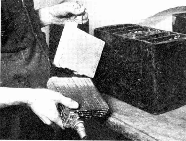
Fig. 6.—PLACING THE POSITIVE GROUP OF PLATES INSIDE THE NEGATIVE GROUP.
