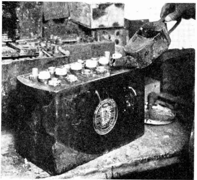
Fig. 7.—USING A METAL CONTAINER WITH A LEADING-OUT SPOUT FOR APPLYING THE SEALING COMPOUND.
