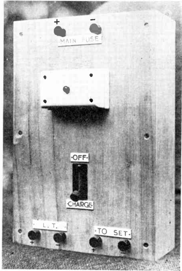
Fig. 5.—FRONT VIEW OF L.T. CHARGING SET TO OPERATE FROM D.C. MAINS.
