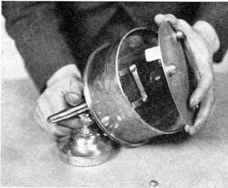
Fig. 11.—ASSEMBLING THE COMPONENTS OF THE ELECTRIC KETTLE. Showing how the base plate is fitted in position.
