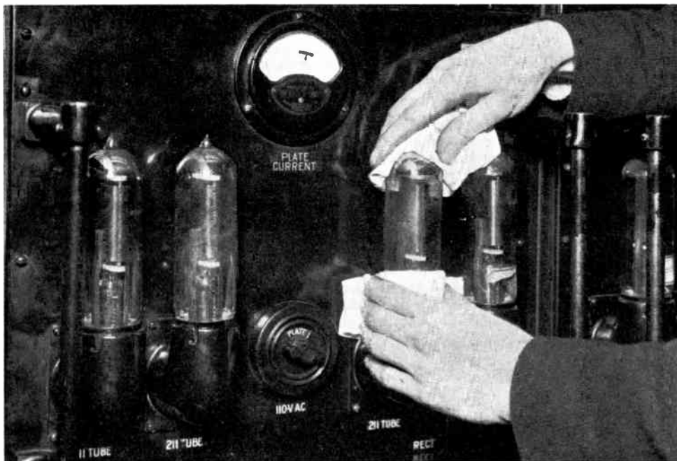
Fig. 11. —HOW TO HANDLE THE 211E VALVES WHEN CHECKING THEIR EMISSION. As these valves get very hot it is advisable to use a rag or cloth as indicated.
