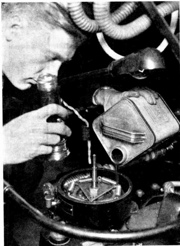
Fig. 17.—FILLING 703 DRIVE WITH OIL.
