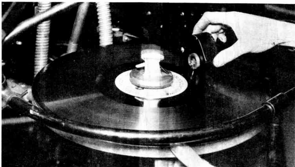
Fig. 1. —How to Start the Reproducer on the Record.
