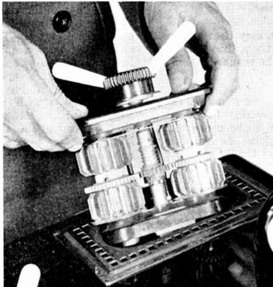
Fig. 4.—PLACING SPARK GAP IN POSITION.
