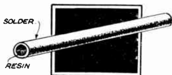
Fig. 7.—RESIN CORED SOLDER, By means of which the solder is melted on to the job and the flux automatically applied in about the correct amount at the correct place.
