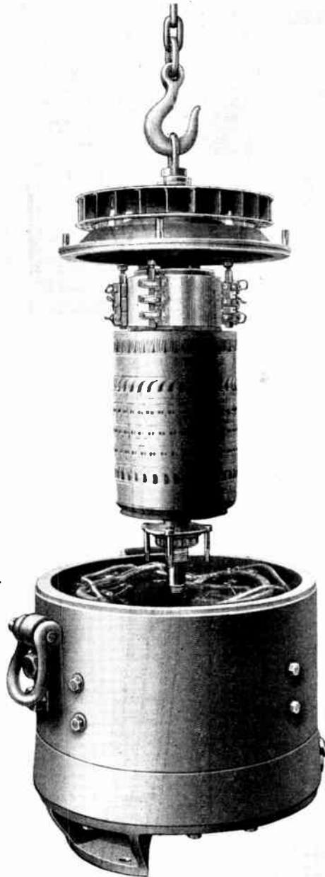
Fig. 19.—METHOD OF REMOVING ARMATURE OF MOTOR ILLUSTRATED IN FIG. 17.
