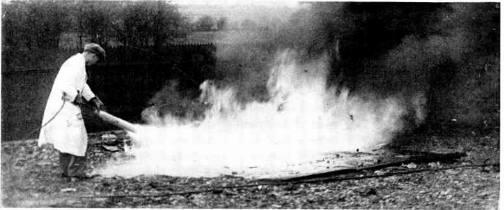
Fig. 1. —EXTINGUISHING AN OIL FIRE WITH CARBON DIOXIDE GAS.
