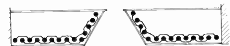
SWITCH CONTROLS FOR WINDOW REFLECTORS. Correct arrangement for even lighting with alternate lamps.
