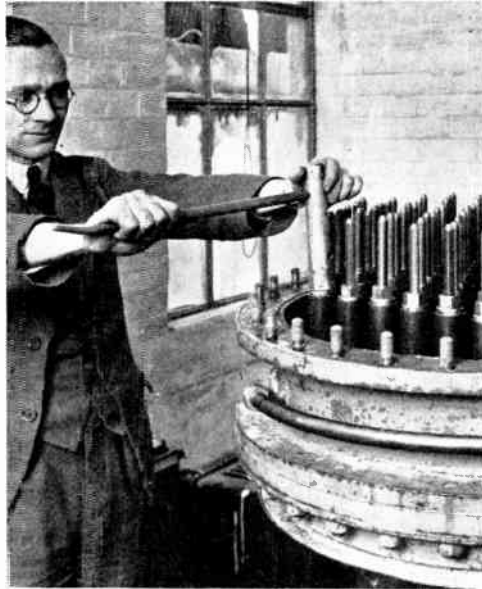
ADJUSTING FILTER PACK COMPRESSION OF GRID SCHEME FILTER.
