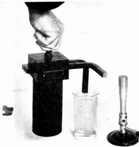
Fig. 3.—THE DEMONSTRATION. After a short time it is found that the whole apparatus can be lifted bodily owing to the magnetic effect between the armature and plate.
