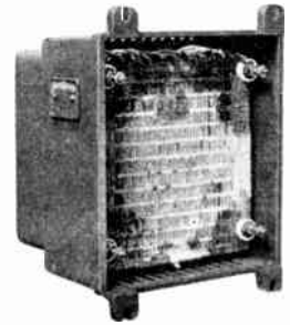
THE MOTOR STARTER OR SHUNT REGULATOR COMPLETED.
