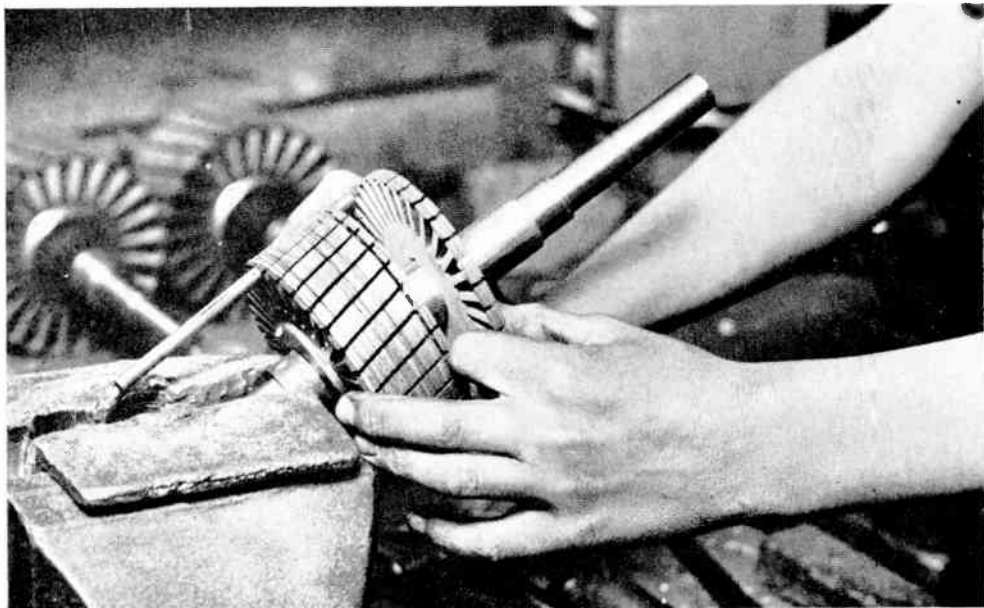
ASSEMBLING THE ARMATURE STAMPINGS.
