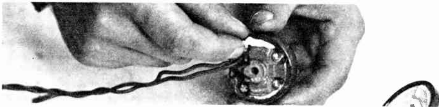
REPLACING THE ASBESTOS CORD IN POSITION.
