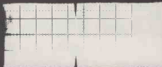
A trace showing the sudden loss of output caused by a scratch on the disc surface. This is known as dropout.
