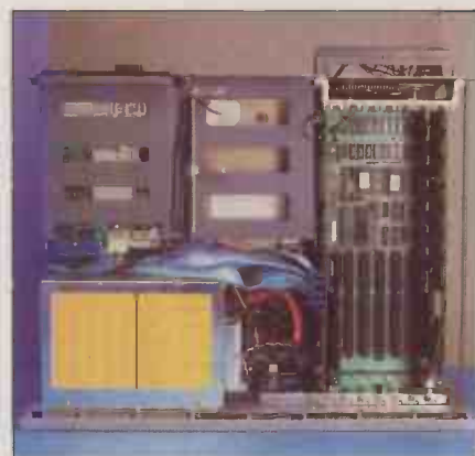
Above: The Wyse PC-286 is solidly built. Left: The sliding cover for disc drives on the Wyse protects against dust.
