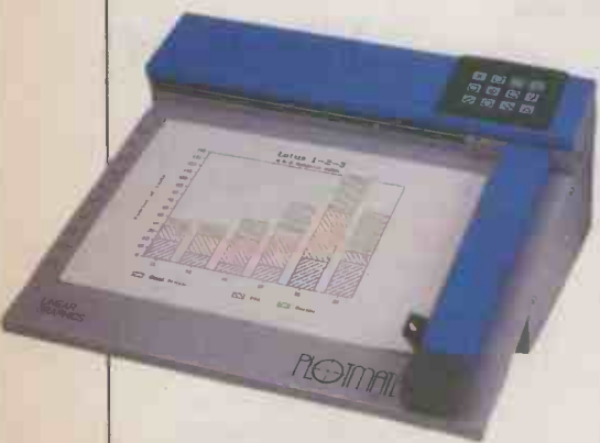
The flat-bed Plotmate from Linear Graphics of Rochford, Essex is cheap but for multi-colour plotting the pen must be changed by hand.
