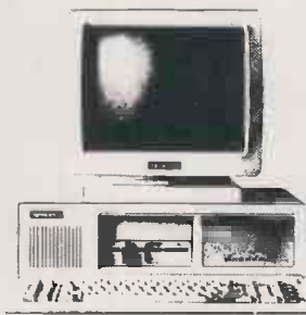
PCA, THE TANDON AT Intel 80286 6.8 Mhz, 1.2 Mb FDD, 640 KByte main memory, 30 MByte Fixed Disk, 14" Tilt/Swivel Hi Res monitor, keyboard, MSDOS.
