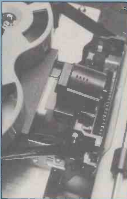
The daisywheel rotates to position the required character under a hammer, which strikes it against an ordinary typewriter ribbon.
