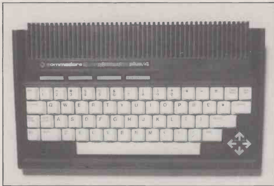
The Plus-4's switch-like function keys are easy to use, as are the neat compass-point cursor-control keys.
