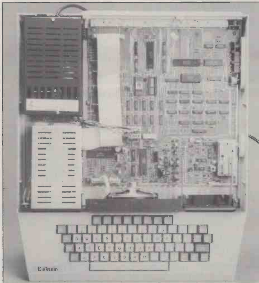
There is space inside the Einstein's casing for a second disc drive.
