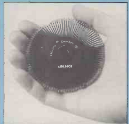
A typical daisywheel has 96 characters mounted on the end of flexible stems.
