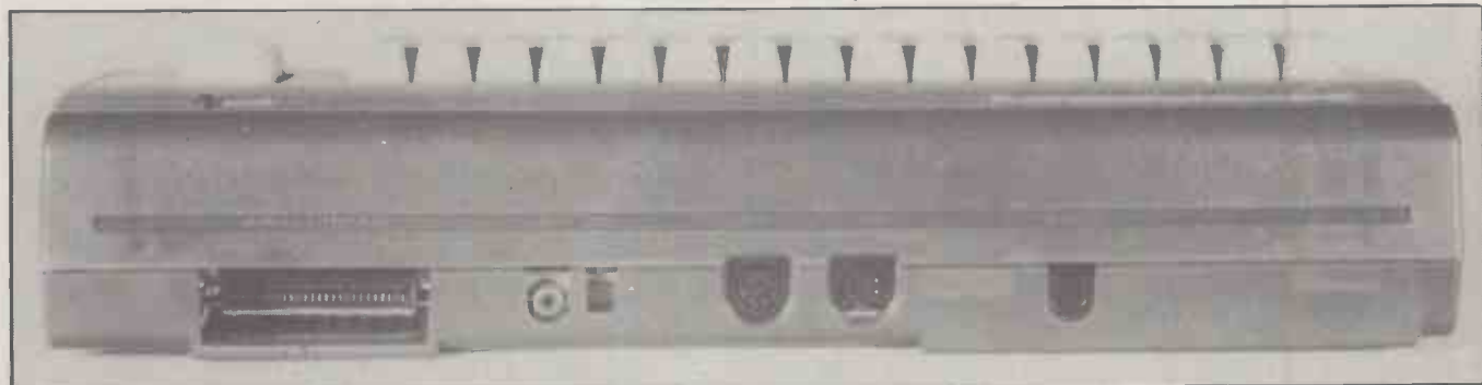
Like the Plus-4, the 16 has an expansion socket incapable of taking extra memory, and a standard Commodore serial port.
