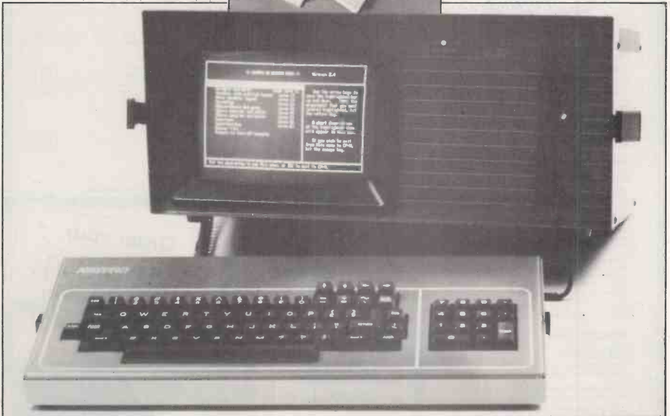
The Kaypro comes with a generous quantity of software installed on the 10MByte Winchester, including WordStar and three Basics.
