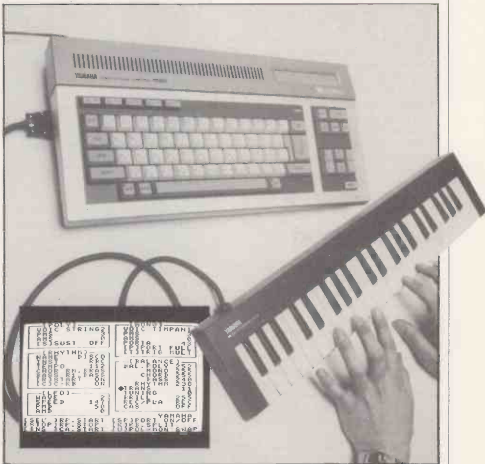
The 3 1/2-octave music keyboard plugs into the synthesiser; the software control panel is displayed on the screen by typing Call Music from Basic.
