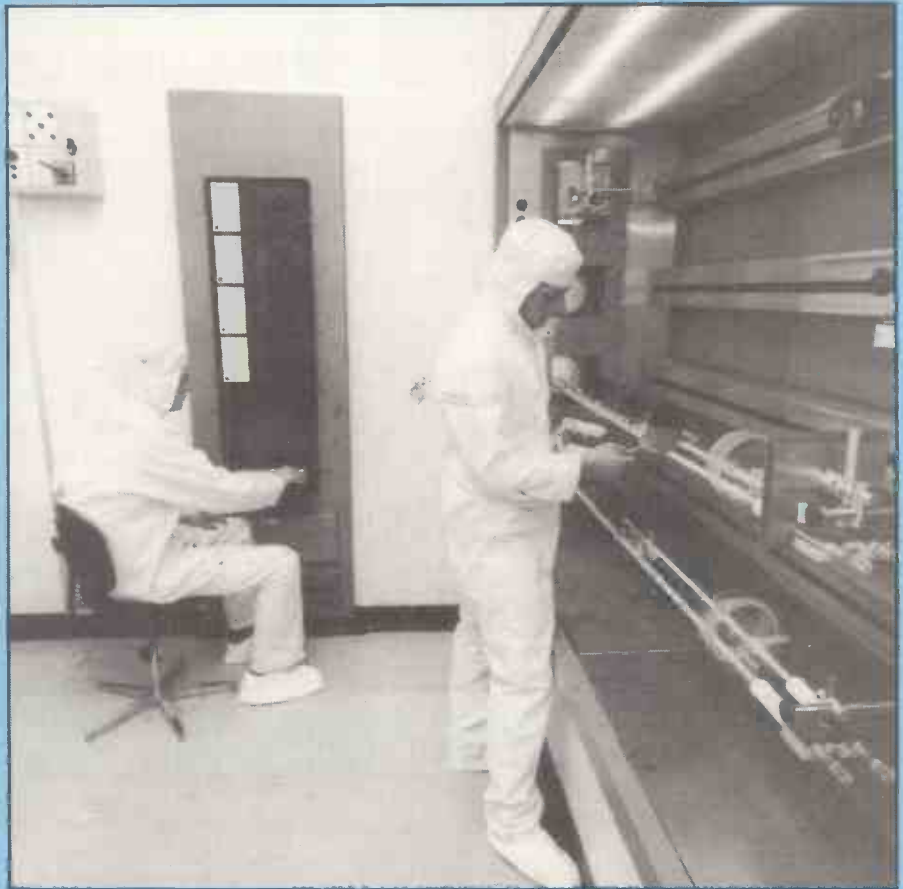
Preparing silicon wafers at Ferranti for ULA chips, key elements in cheap home micros.
