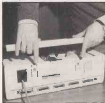
Terminals are connected via RS-232 links; a Centronics interface is also provided.
