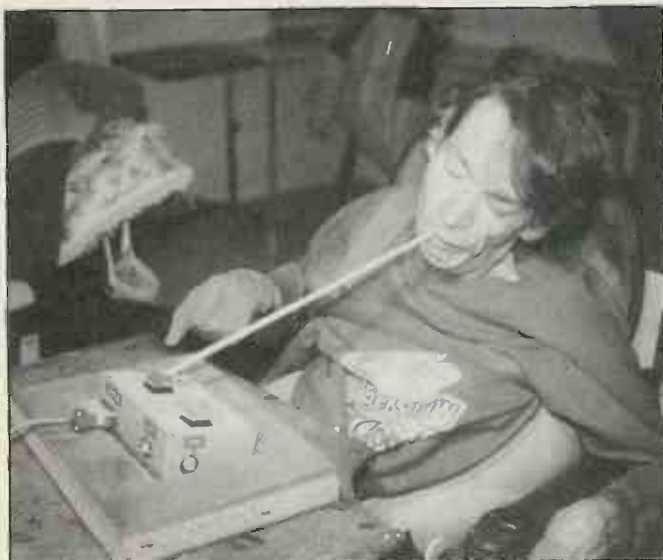
An alternative mouthstick controller allows MacApple to be used by operators without the need to exercise fine control of the limbs.
