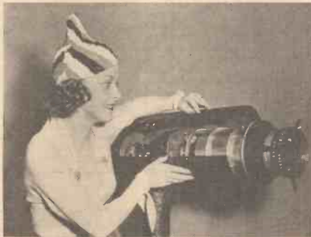
A view of the latest American television receiving cathode-ray tube, which, like sets that have already been demonstrated in this country, produces pictures up to two or three feet in size by means of optical projection on to a screen from the very bright picture produced on the end of the tube.
