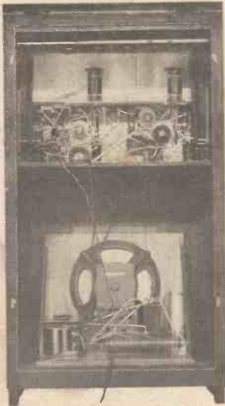
The power pack and loudspeaker are arranged as a separate unit below the receiver itself.
