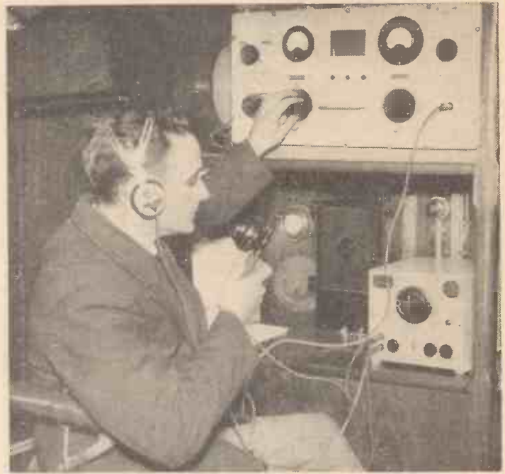
This transmitting and receiving set has recently been installed in the Clacton-on-Sea lifeboat to enable her to keep in touch with her home station when called out to ships in distress. The installation is operated by the first engineer, Mr. W. C. Harding.
