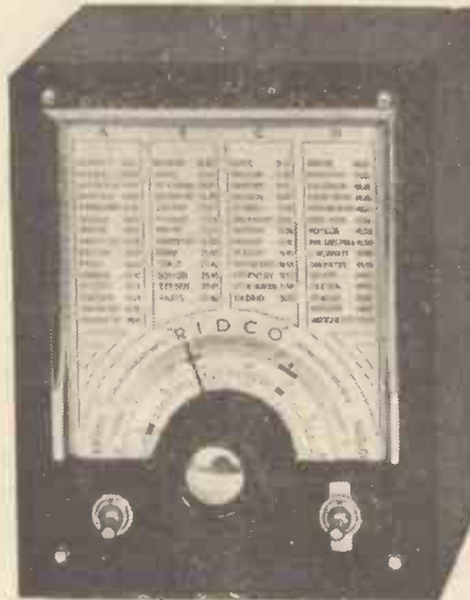
The latest Ridco "Ranger" short-wave converter. It tunes from 12-60 metres in two wavebands. Further details were given in last week's "Radio Bulletin."
