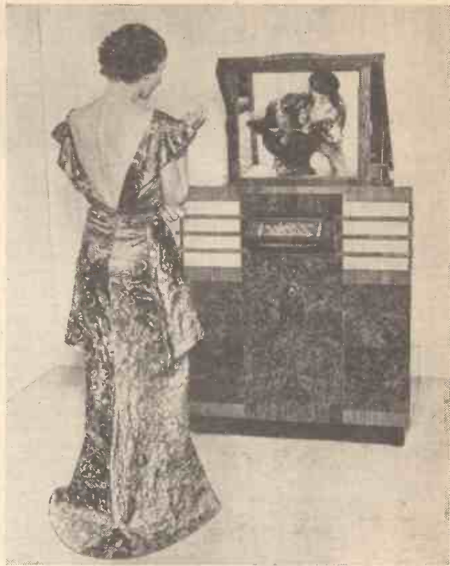
The Philips big-screen television receiver in which a small cathode-ray tube projects a brilliant picture on to a flat screen measuring 20 in. x 16 in.
