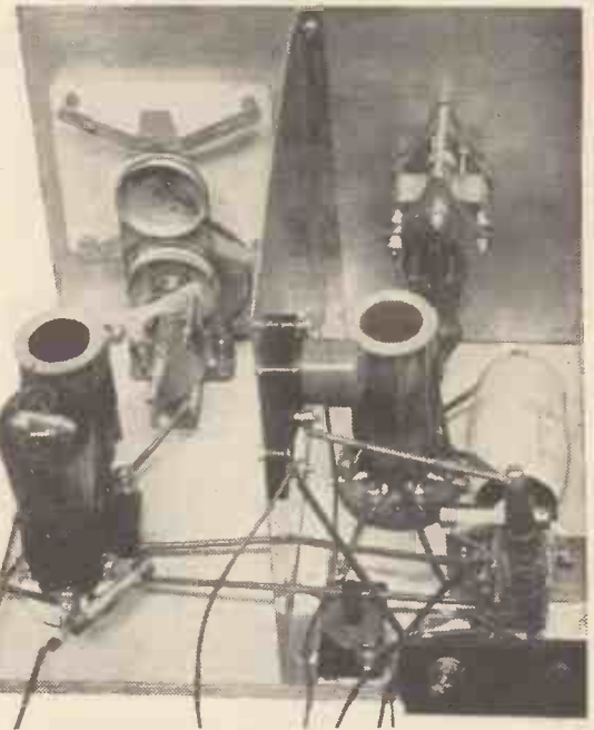
The oscillator stage is separated from the mixer and reaction stages by a vertical metal screen. The panel is of aluminium, while the baseboard is metallised.
