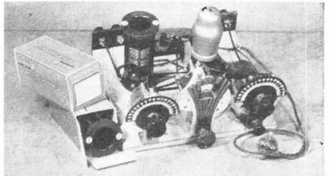
The New Times Sales Combination Short-Wave Kit Set. It can be used as a single-valver or an adaptor-converter.
