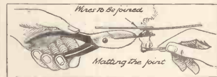
How the wires are applied to the solder for joining together.
