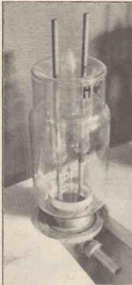
One of the large high-frequency "tubes" used in the R.C.A. television transmitter in the Empire State Building, New York. Note the inlet point for the water used to keep the anode cool when the valve is working
