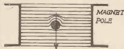
A conductor in a magnetic field tends to move in a certain direction.
