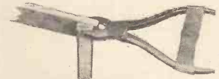
Pliers are useful for holding pieces of wood in position for gluing, if arranged like this.
