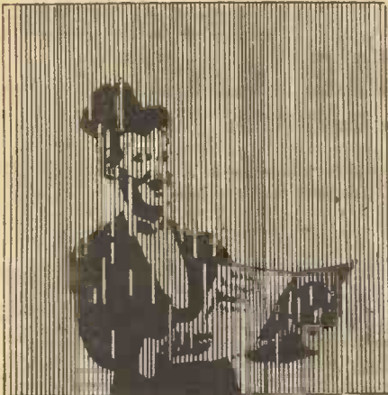
Man-made static looks somewhat like snow. It is shown in this sketch on a vertically scanned picture.
