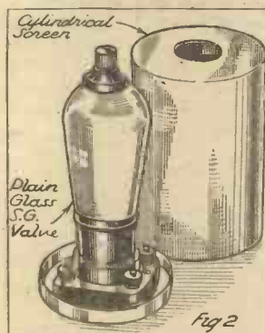
A good method of screening when a non-metallised valve is used.
