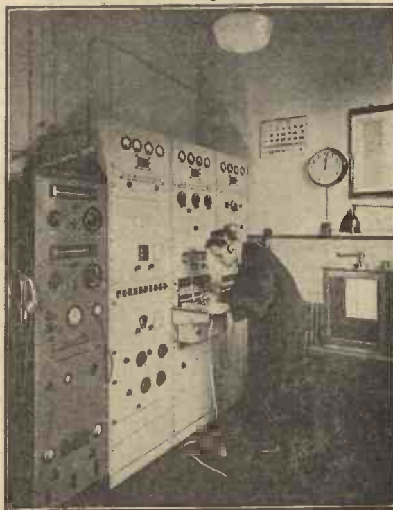
The frequency measurement room at the B.B.C. checking station at Tatsfield. The engineer is checking the rate of the crystal frequency standard against Rugby time signals.
