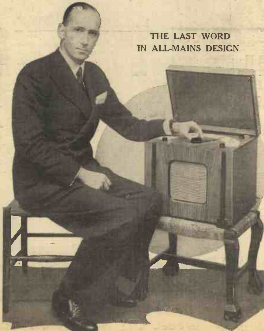
Mr. Scott-Taggart with the extremely handsome A.C. S.T.700. As can be seen, the auto-dial and controls are neatly arranged immediately beneath the cabinet lid, while the loudspeaker is "built-in."
