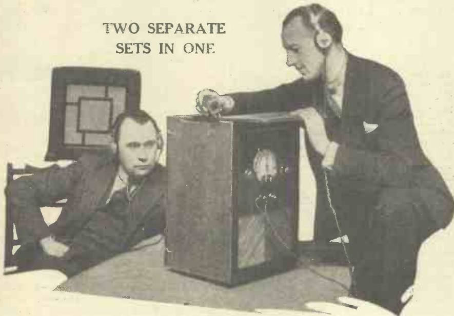
Mr. G. T. Kelsey is here seen inserting a short-wave coil in the "Silver King," as explained on page 177, while the broadcast side is actually working.
