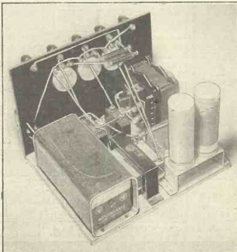
A metal rectifier is employed in the H.T. unit, and it can be seen to the left of this photograph. Note the three potentiometers on the panel for the variable H.T. taps.
