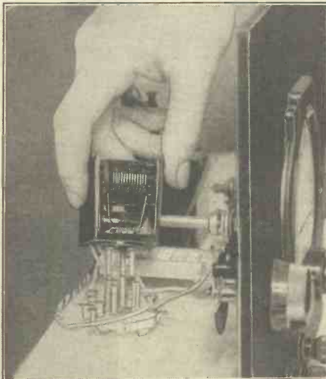
A surprisingly large range of short waves is covered by the "Silver King," and the band is changed simply by changing one plug-in unit. This is done through the lid of the cabinet, and does not interfere with medium- or long-wave reception in the least.
