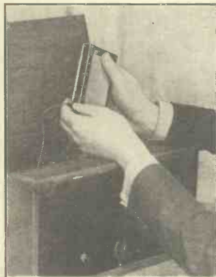
A grid-bias battery will not last for ever. After nine months—and even before—it should be tested for voltage. Here is one being removed from a set after 15 months' use. The set was faulty, and no wonder, for the grid-bias battery gave only half its proper voltage.
