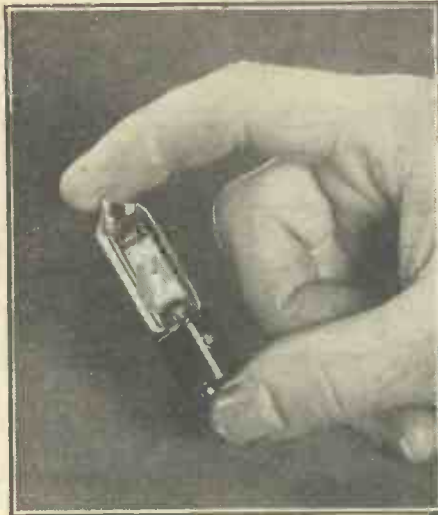
REMARKABLY SMALL. One of the Hivac Midget valves.
