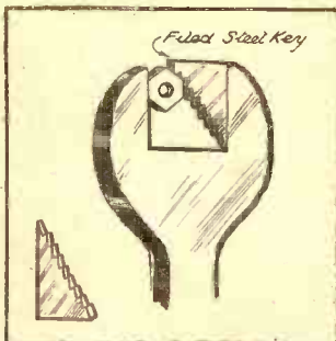
Different sized nuts can be handled with this spanner.
