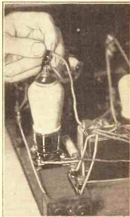
The S.G. valve, in the grid and anode circuit of which the Bifocal coils are placed, is here shown with an anode connector being placed in position. It is this valve and its associated circuits that ensure the set its magnificent range of reception.
