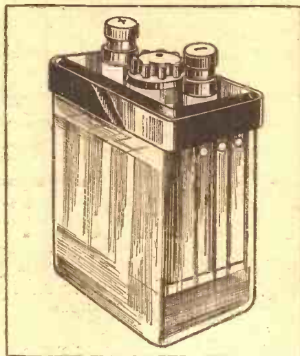
Some batteries have three beads, to indicate the various degrees of charge. By enabling the listener always to keep his accumulator in tip-top condition these beads greatly increase the life of the battery.
