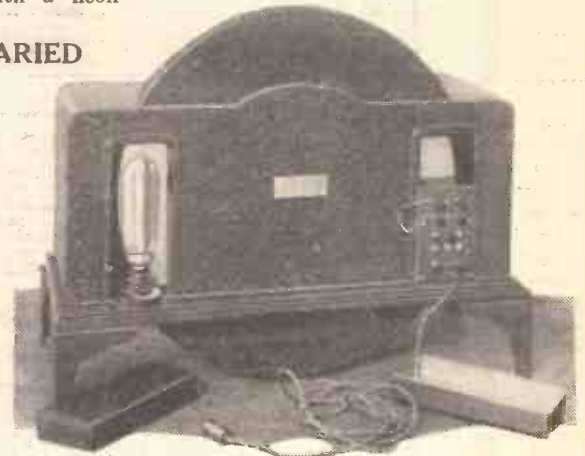
This back view of a Baird Televisor shows a lamp of the neon type in position. Unlike the huge affair shown in the adjacent column, it is suitable for home use. When the television receiver is in action, the cover is replaced over the lamp, to prevent escape of light from the back, and the terminals also are screened off on account of the high voltages used.
