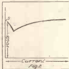
Fig. 2 illustrates the voltage regulation possible with the use of a stabiliser, while Fig. 5 shows the arrangement of the "gaps" in the new "divider."
