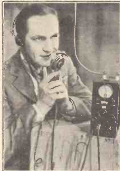
A short-wave transmitting set, weighing only twenty-five pounds, in use at an American film studio. It is employed on large "sets," where its portability is of great advantage and saves the fixing of numerous points for "line" telephones.
