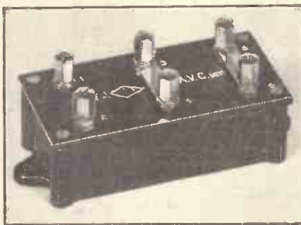
There are several makes of commercial Automatic Volume Control units on the market. All of these are self-contained, making use of a Westector for the rectification of A.C. as explained by our Chief Radio Consultant. Readers who think of converting their own receivers to use A.V.C. should remember that considerable high frequency amplification is necessary to ensure the satisfactory working of such a control, and it should not, as a rule, be incorporated in a set having less than two H.F. stages. Circuits incorporating A.V.C. have been published from time to time in "POPULAR WIRELESS."
