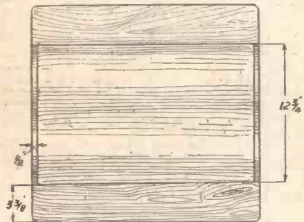
The top of the cabinet is provided with a domed piece, as indicated here, which covers the cathode-ray tube.
