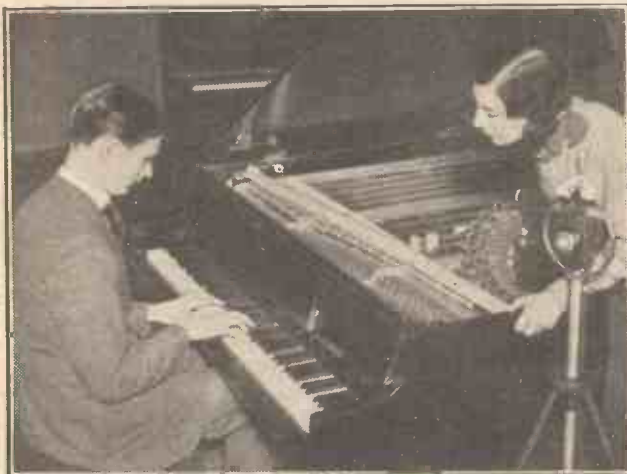
The piano, with its wide band of frequencies, has always been a test of good quality reception. This is the Neo-Bechstein, in which the string vibrations are picked-up by microphones, amplified, and reproduced by a loudspeaker.
