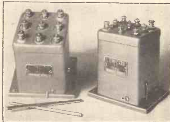
The unique Lewcos triple-range coils used in the "No-gap" Three are the outcome of these, which are two of the experimental types made during the development work. The production coils are not quite so tall, and the wavechange spindles come through higher up.
